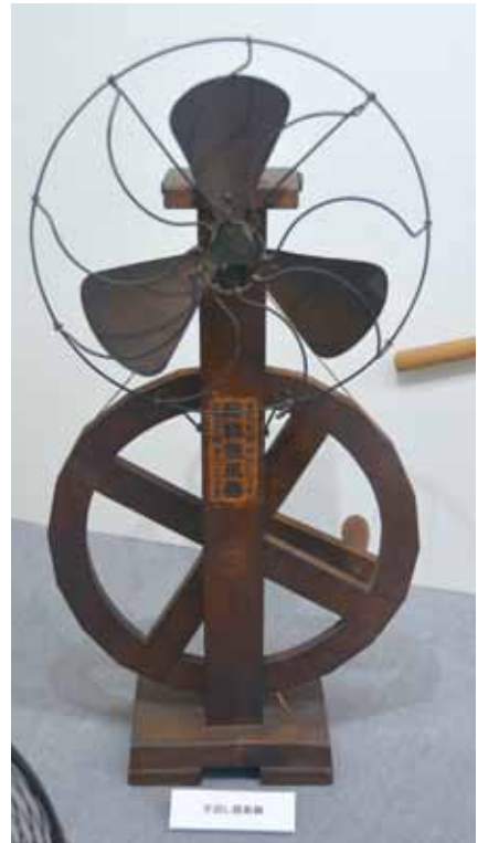
Fan This is a manual fan. When turning the lever, the blades of the fan rotate.
